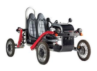
Light electrical quadricycle two-seater Four wheel steering on independent suspensions Reverse gear Foldable rear rack for bags, equipment etc (optional extra)
