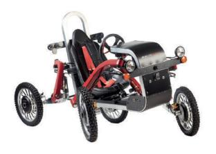
Light electrical quadricycle one-seater Four wheel steering on independent suspensions Reverse gear
